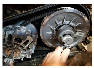
Remove drivers side rear wheel. Remove cover bolts and plastic cover to expose CVT clutch system.
