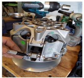
Make sure the governor and sliding sheave are **marked for index**.
