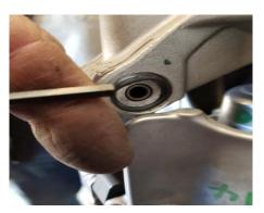
temporarily fold the flyweight lever arms to be out of the way for removal of the primary spring.
